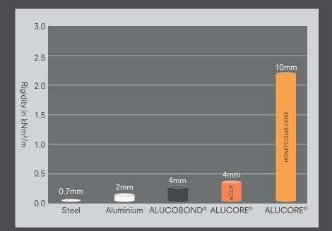
The graph illustrates the rigidity of different materials while keeping the weight identical ~5Kg/sqm.
