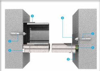
Self-supporting ceiling perimeter to wall intersection (case 2)
