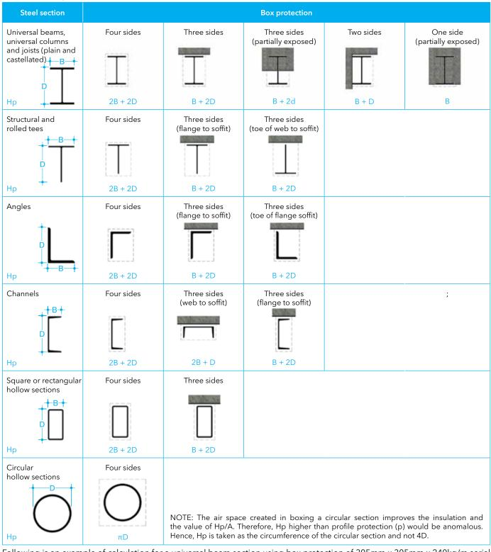
Following is an example of calculation for a universal beam section using box protection of 305mm x 240kg/m serial size to be encased on three or four sides when A = 305.6cm<sup>2</sup>, B = 317.9mm, D = 352.6mm, t = 23mm.
