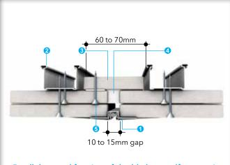
Parallel to steel framing of double layer self-supporting ceilings
