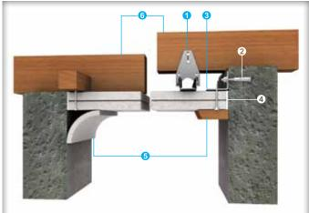
Suspended ceiling perimeter to wall intersection (for timber floor protection)
