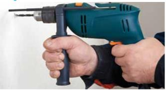
Drilling can be carried out either by hand drill or any conventional power drill with or without dust extraction. For best results, the boards should be firmly supported behind the location of the holes. Generally when working on PROMATECT® 100 boards, the use of drills with point angles of 60° to 80° rather than the more usual 120° type, are preferable and more efficient.
