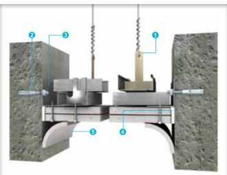
Suspended ceiling perimeter to wall intersection
