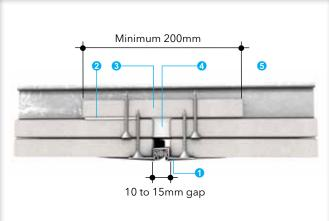
Perpendicular to steel framing of double layer self-supporting ceilings
