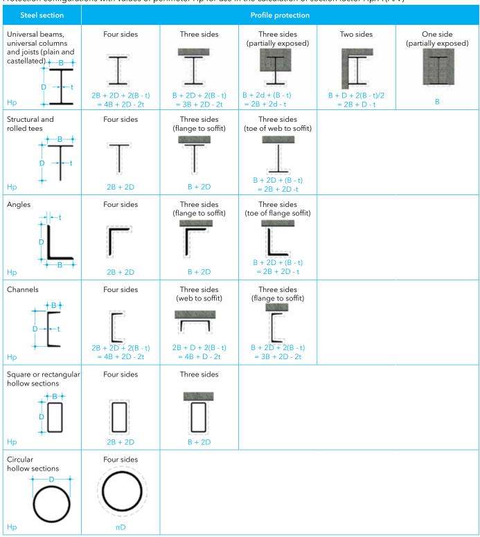
Following is an example of calculation for a universal beam section using profile protection of 305mm x 305mm x 240kg/m serial size to be encased on three or four sides when A = 305.6cm<sup>2</sup>, B = 317.9mm, D = 352.6mm, t = 23mm.
