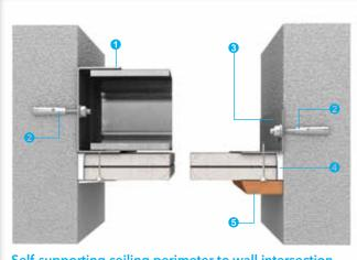
Self-supporting ceiling perimeter to wall intersection (case 1)
