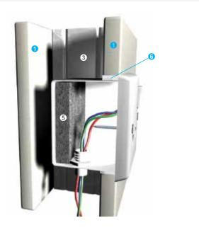
NOTE: For fire resistant walls, steel electrical switch boxes should be employed to avoid degrading fire performance of the wall system
