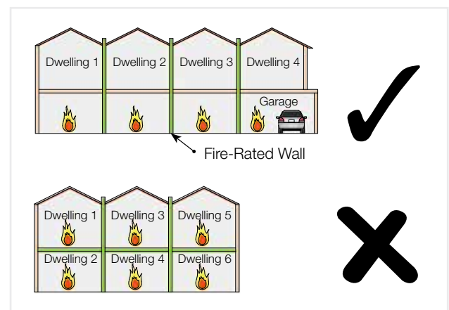
FIGURE 1 HARDIESMART™ INTERTENANCY WALL SYSTEM TYPICAL APPLICATIONS
