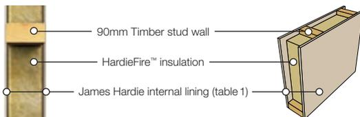
Designed for separating walls between sole occupancies in class 9c buildings; requiring a Fire Resistance Level (FRL) of up to 1 hour and an acoustic rating  $R_w \leq 45^{**}$ . This integrated solution will also provide you with excellent energy efficiency and bracing performance.
