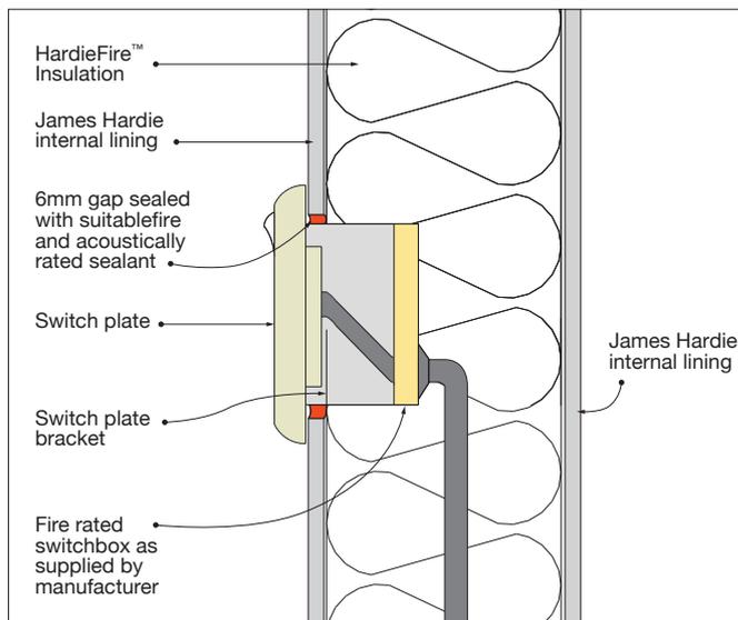
FIGURE 7 FIRE-RATED SWITCH PLATE OR GENERAL POWER OUTLET (GPO) ELEVATION
