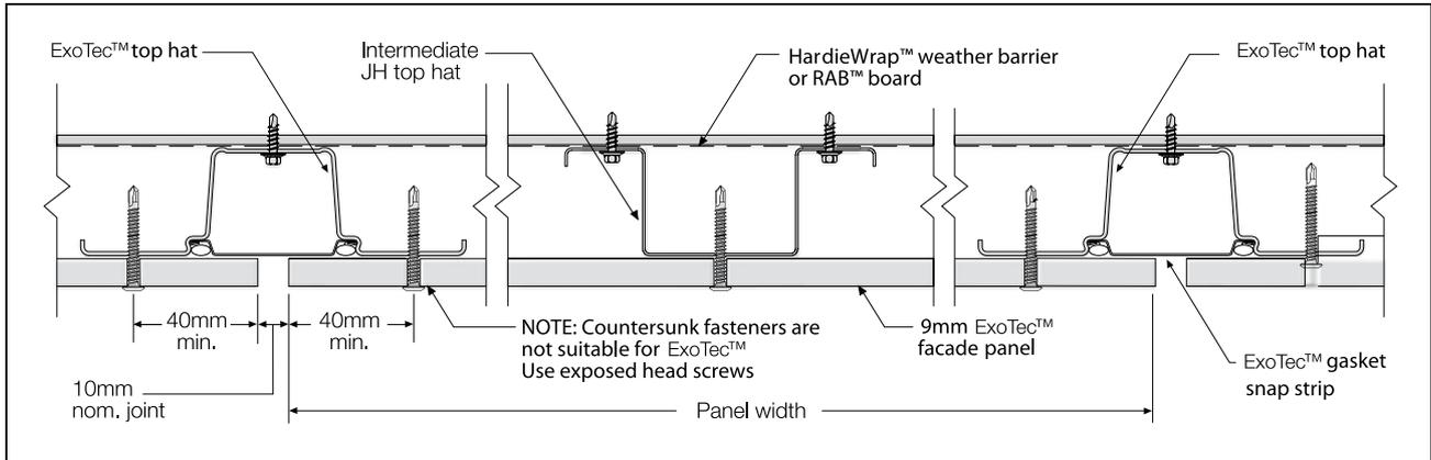
TOP HAT AND PANEL FIXING DETAIL FOR EXOTEC™ PANELS
