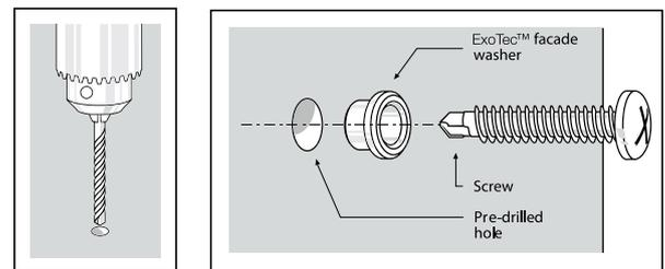
DRILL CLEARANCE HOLE & WASHER AND SCREW INSTALLATION
