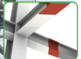
Intumescent Paint To Structural Steel
