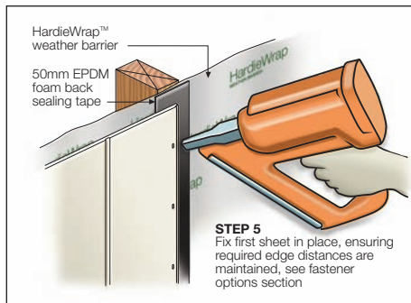
FIGURE 7 FIX FIRST SHEET
