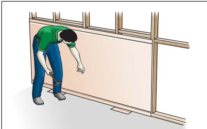
FIGURE 4 FIXING FIRST SHEET
